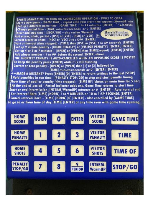
PENALTIES — When PENALTIES are inputted the displays will "flash" this indicates to the timekeeper that the scoreboard is ready to accept the information from the control panel. If an error has been made the information can be corrected during the flashing mode. The display will flash for 5 secs.
